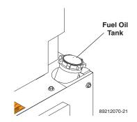
**STEP 8:** Fill fuel oil tank. Do not confuse gasoline and fuel oil tanks. Keep proper fuel in proper tank.
