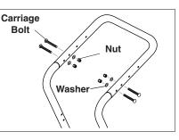
**STEP 2:** Insert the carriage bolt through the holes from the outside of the unit and attach a nut from the inside of the machine. Tighten nuts.
