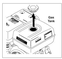
STEP 3: Fill gas tank with unleaded gasoline. Do not use leaded gasoline.
