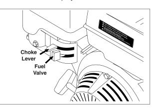
STEP 6: Rotate the fuel shut-off valve to the "On" position. Slide the fuel valve lever to the "ON" position. When the engine is not in use, leave the fuel valve in the "OFF" position.
