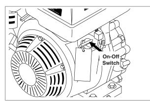
**STEP 8:** Turn the engine switch to "On" position.
