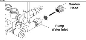
STEP 9: Connect the garden hose to pump water inlet. Inspect inlets. CAUTION: Do not run the pump without water or pump damage will result.
