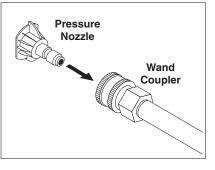
**STEP 5:** Pull the spring-loaded collar of the wand coupler back to insert your choice of pressure nozzle.
