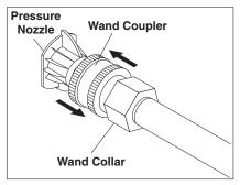
**STEP 6:** Release the coupler collar and push the nozzle until the collar clicks. Pull the nozzle to make sure it is seated properly.
