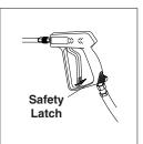
STEP 6: Disconnect the high STEP 7: Engage the pressure hose from discharge spray gun safety lock. nipple.
