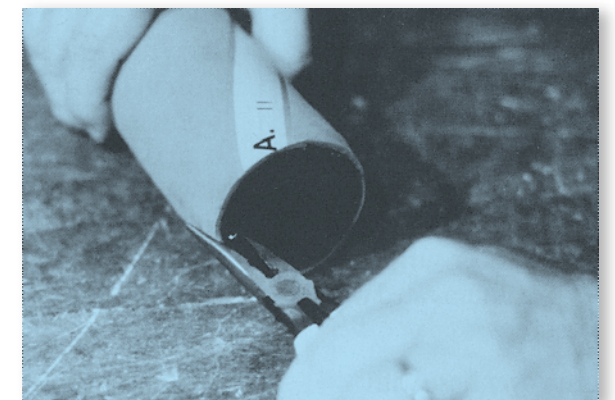
Pinching the staple into the tube wall.
